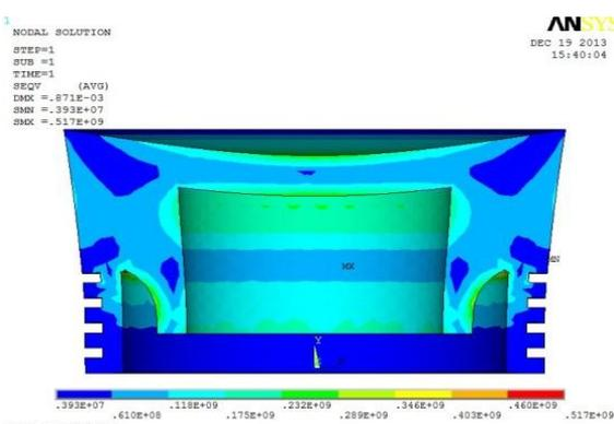
Figure 9: Coupled Thermal-Mechanical stress on the piston
