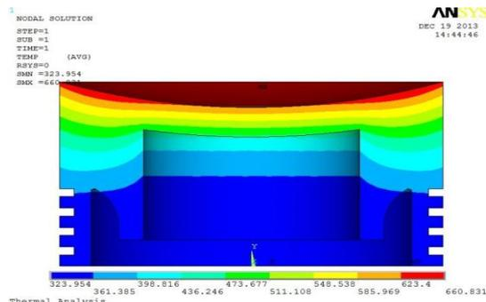
Figure 3: Temperature distribution over the piston.
