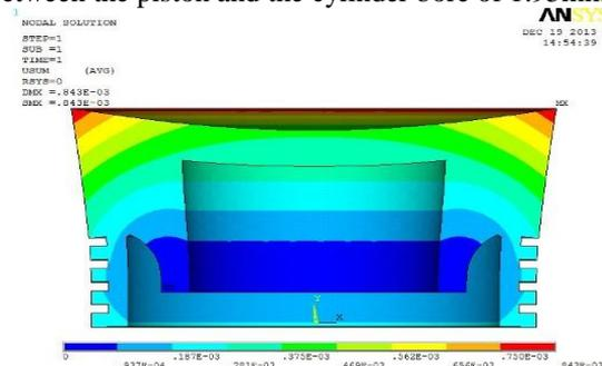
Figure 4: Piston deformation under thermal load
