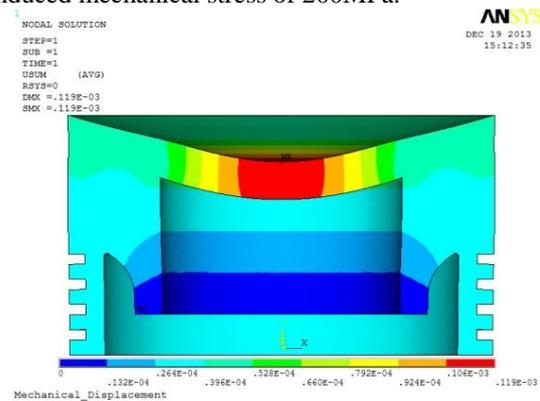
Figure 6: Piston deformation under mechanical load
