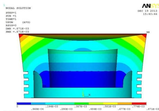
Figure 8: Piston deformation under coupled Thermal-Mechanical load
