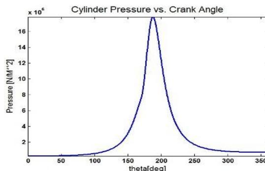
Figure 2: Pressure variation with crank angle
