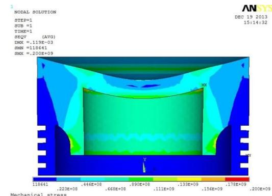
Figure 7: Mechanical stress on the piston
