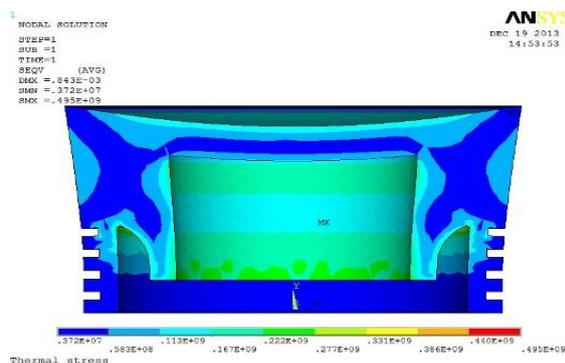
Figure 5: Thermal stress on the piston
